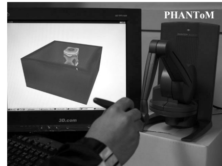
Fig. 2. Field distribution map and haptic interface (PHANToM).
