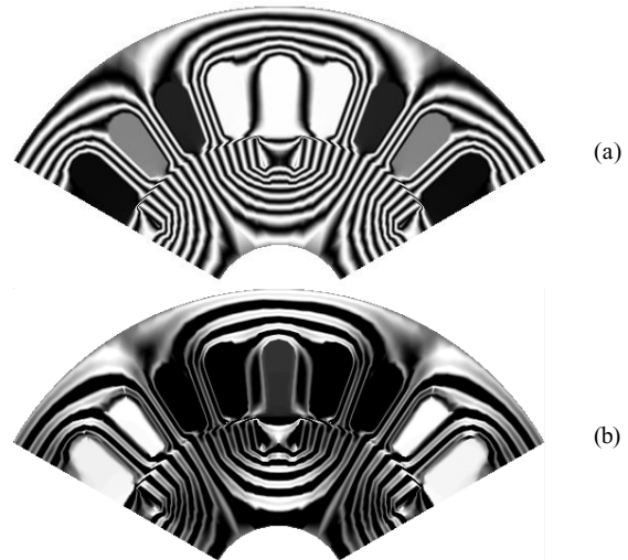
Fig.4. SMP images of the magnetic field in a PM motor
