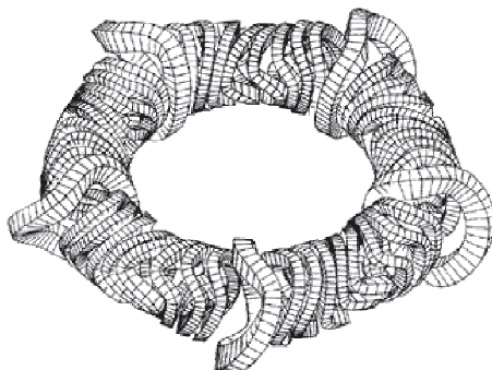
Fig. 1. Sketch of the non-planar coils of the Wendelstein 7-X stellarator (courtesy of IPP)
